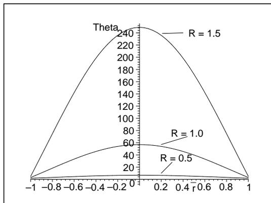
Figure 3: Temperature distribution profile ( $P = 7.1$ )
