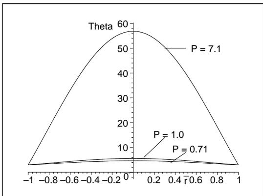
Figure 2: Temperature distribution profile ( $R = 1$ )
