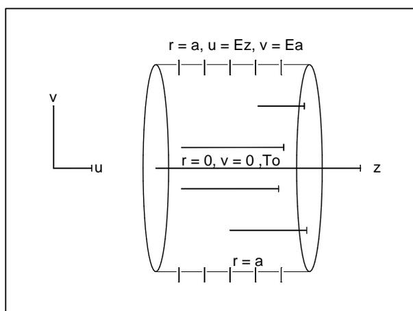
Figure 1: Wall driven steady flow in a uniformly porous tube.
