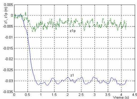
Figure 9: Displacement of abut mass and front wheel center of the vehicle S
