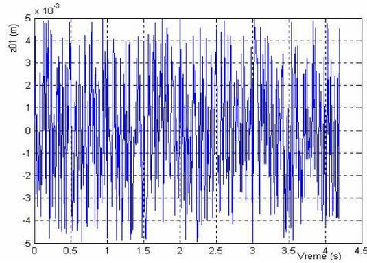
Figure 3: Function of uneven road in the points of contacts of front wheel and the ground
