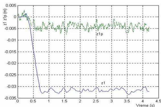
Figure 5: Displacement of abut mass and front wheel center of the vehicle F
