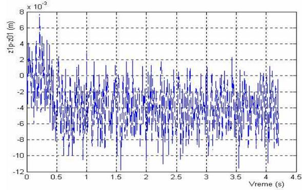
Figure 7: Difference of displacement of wheel center and uneven road on front axle of the vehicle F
