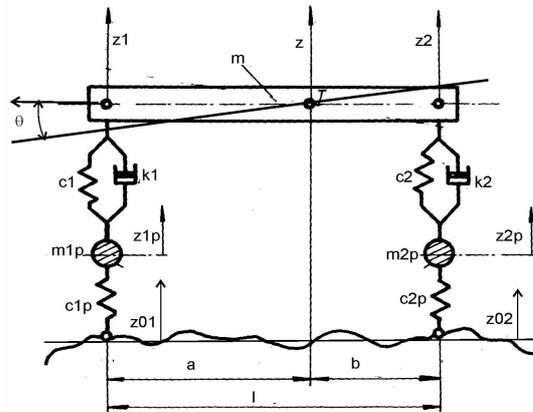
Figure 2: Mathematical model of braking vehicle
