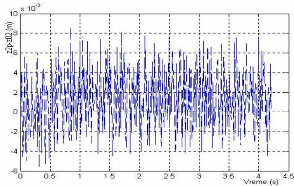
Figure 8: Difference of displacement of wheel center and uneven road on rear axle of the vehicle F
