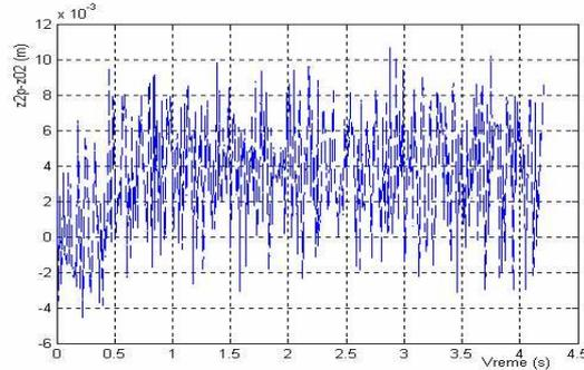
Figure 12: Difference of displacement of wheel center and uneven road on rear axle of the vehicle S
