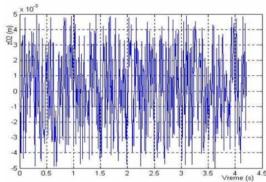
Figure 4: Function of uneven road in the points of contacts of rear wheel and the ground
