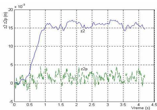
Figure 6: Displacement of abut mass and rear wheel center of the vehicle F
