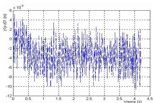
Figure 11: Difference of displacement of wheel center and uneven road on front axle of the vehicle S
