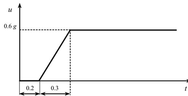
Figure 1: Diagram of vehicle slowing down
