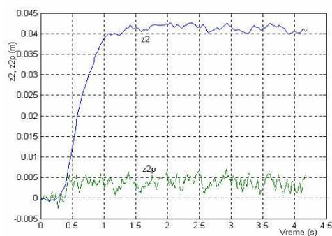
Figure 10: Displacement of abut mass and rear wheel center of the vehicle S
