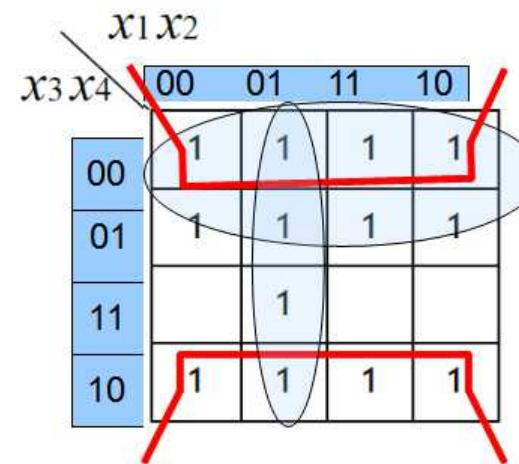
$$f = \overline{x_3} + \overline{x_4} + \overline{x_1}x_2$$
