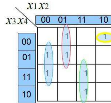
$$f = \overline{x_1} \overline{x_2} x_4 + \overline{x_1} x_2 \overline{x_3} + x_1 x_2 x_3 + x_1 \overline{x_2} \overline{x_3} \overline{x_4}$$
