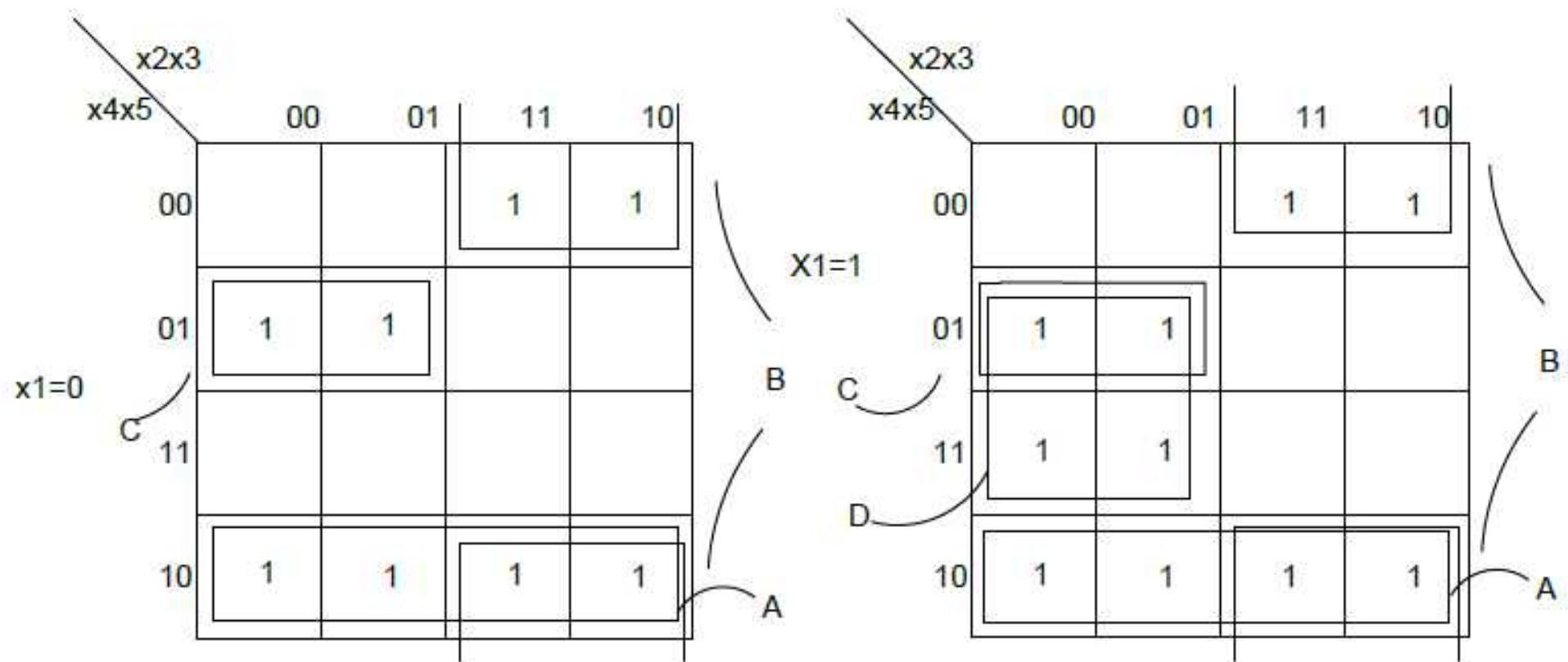
$$f = x_4\bar{x}_5 + x_2\bar{x}_5 + \bar{x}_2\bar{x}_4x_5 + x_1\bar{x}_2x_5$$
